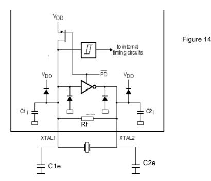
In the Power-down/Stop mode the oscillator is stopped and XTAL1pin is pulled HIGH. The oscillator inverter is switched off to ensure no current will flow regardless of the voltage at XTAL1.
