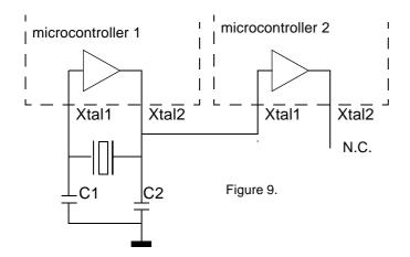
Figure 9. shows this situation when using the standard oscillator circuit. The Xtal2 output (micro 1) is directly connected to the Xtal1 input of the second microcontroller. The Xtal2 output from the second microcontroller remains not connected.
