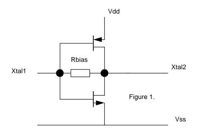
channel transistor. The main difference with a digital inverter stage is an integrated bias resistor (also called: feedback resistor) connected between output and input. This (semiconductor-) resistor feeds back the output voltage to the input which will balance (bias) the stage in its analog working area. In the quiescent situation this will generate a DC- input and output level of about 1/2 Vdd for CMOS devices (For TTL compatible versions it is just a little less).
