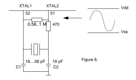
All these circuit examples were tested with a 559 device. They all start oscillating already at about 3 Volts Vdd.
