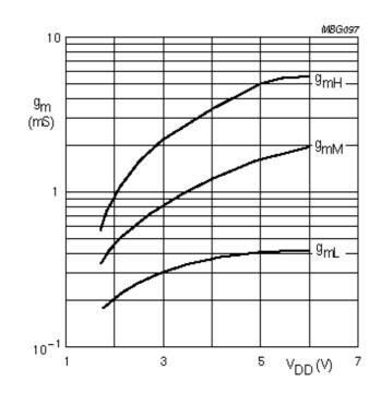
Figure 16:PCF84xx/PCD33xx,Typical transconductance as a function of supply voltage.
