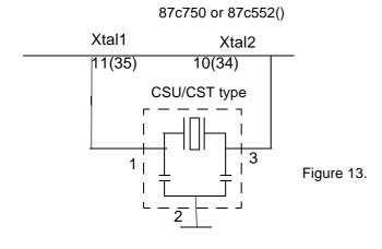
These types of resonators are attractive because of the internal capacitors which saves components and PCBspace in the target system. However it should be considered that when applying these components this eliminates the possibility for reducing the capacitor values which sometimes may be a solution in case the microcontroller is not oscillating.
